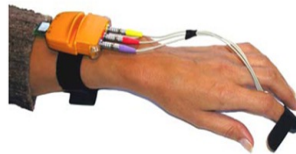
Fig. 4. During the experiment, the module is fastened with Velcro strap to the index finger of the non-dominant hand.
